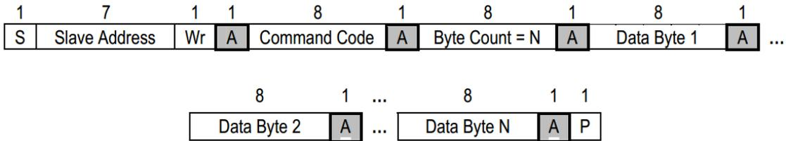
Figure 6-4. Block Write
