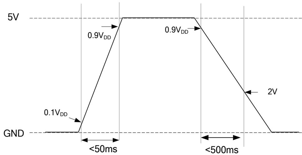
Figure 5-2 Power On/Off Sequence in 5V only mode
