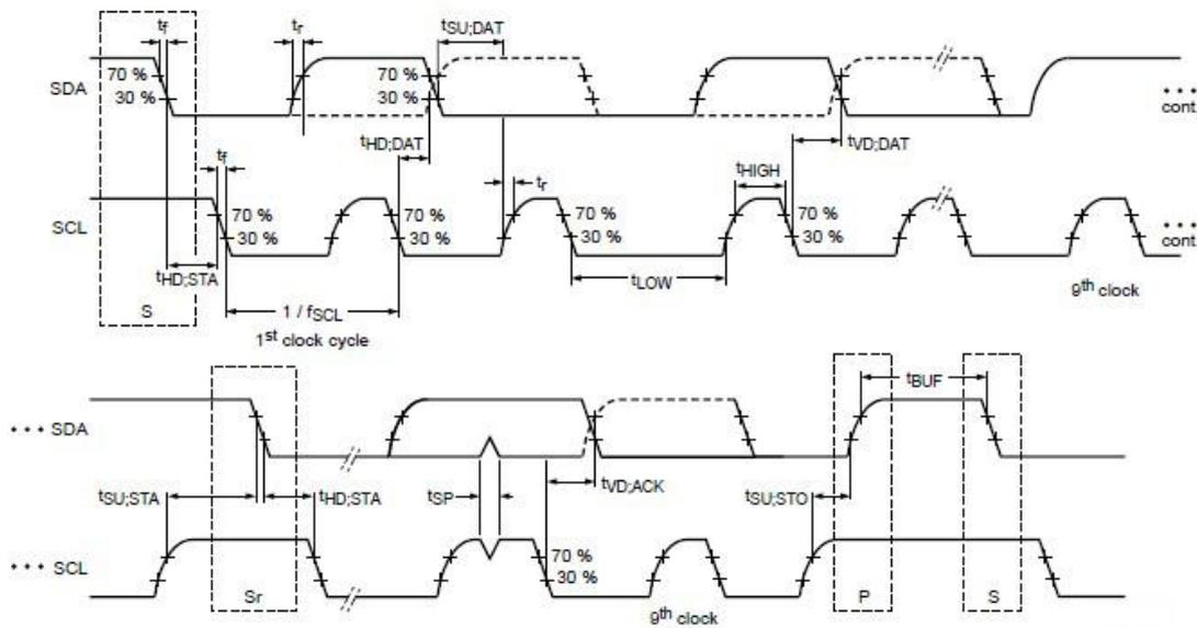
**Figure 7-4 Definition of timing on the I2C bus**
