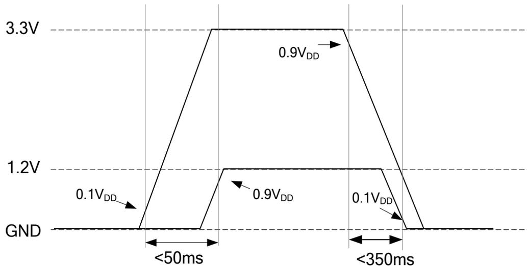
**Figure 5-1. Power On/Off Sequence when 1.2V and 3.3V are provided externally**
